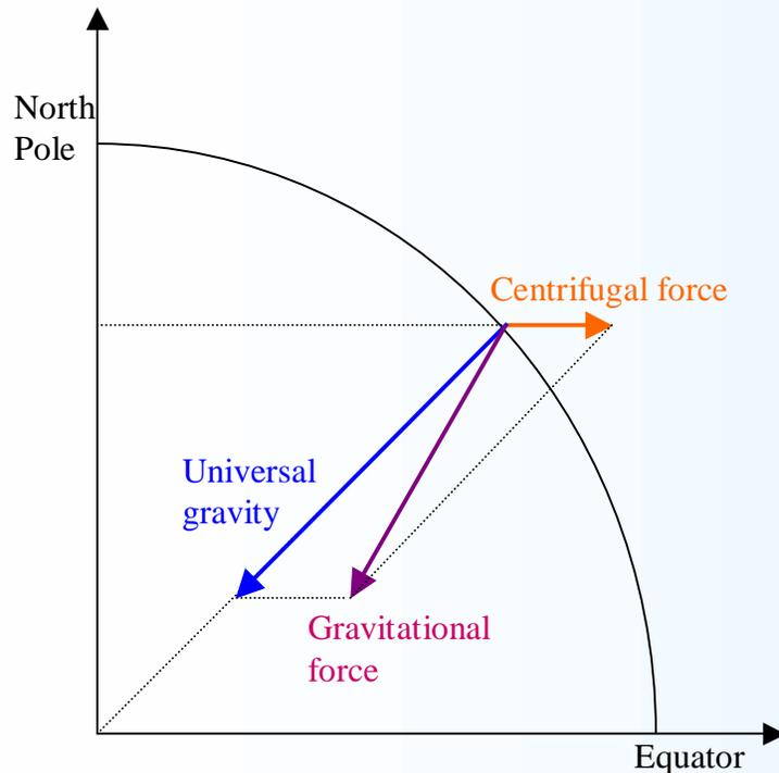
Objects on the earth are constantly subject to the “**universal gravity**,” which attracts them toward the center of the earth, as well as the “**centrifugal force**” caused by the rotation of the earth.
