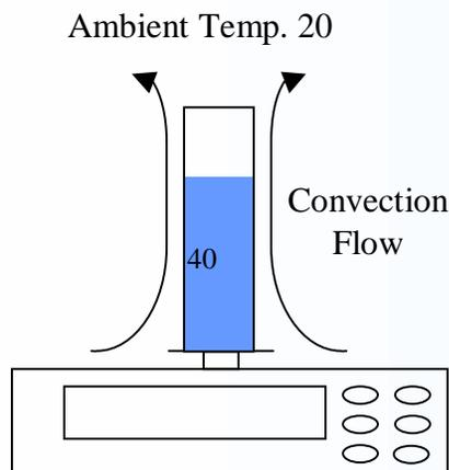
Since this air current will lift up the sample, the balance will display a weight that is **lighter** than the actual sample.
